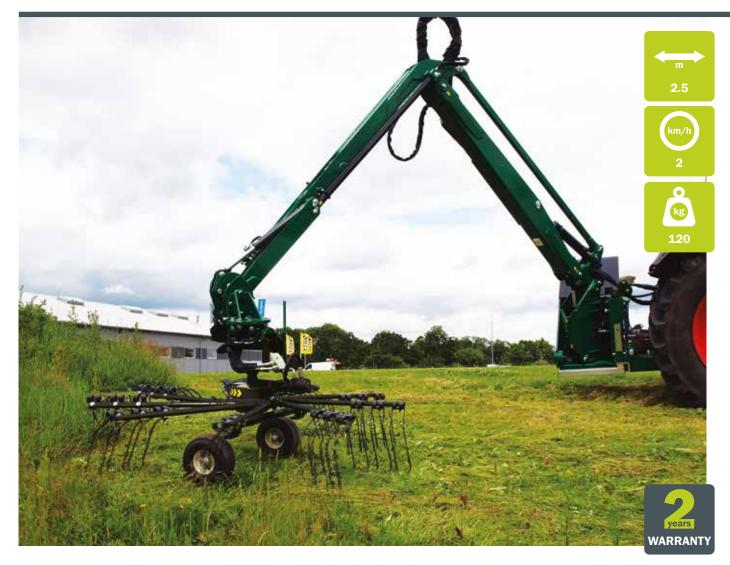
The Rotary Rake KR 250 is the ideal tool to remove cut-off grass from ditches.
