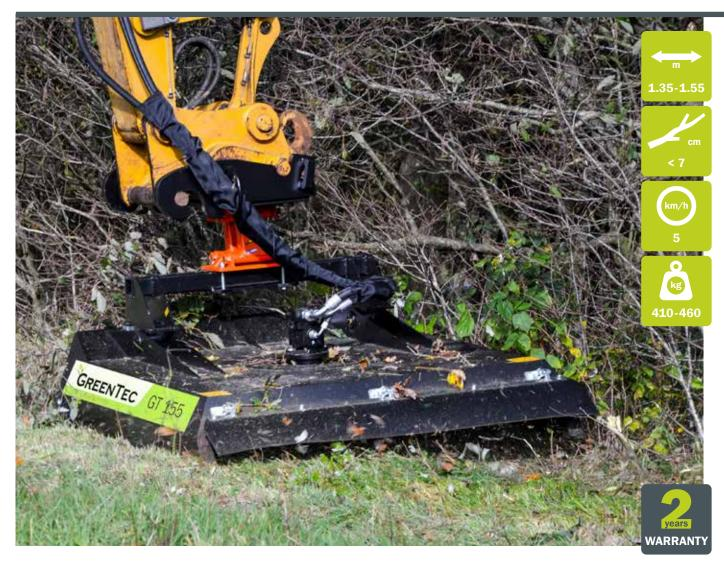
The Rotary Crusher GT 135 & 155 is specially developed for use in extreme conditions with many stones and stumps. It comes with two cutting systems: chains or blades. The chains are used for mowing grass and shrubs in stony conditions. The blades are used for hedge cutting and grass mowing in normal conditions. Both systems are very robust.
